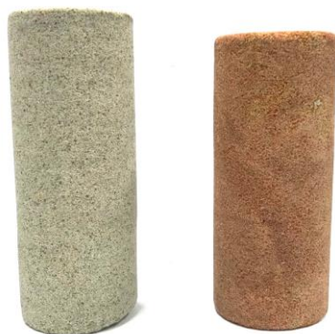
Figure 3.1: Berea (left) and Keuper (right) outcrop rock plugs were used in the experiments.
