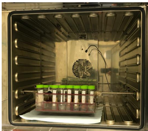
Figure 3.13: A sample holder was mounted on an axis which was connected to an electric motor outside the heating cabinet. The samples were placed in the sample holder and rotated for 24 h at ~35 rpm at RT or 60°C.
