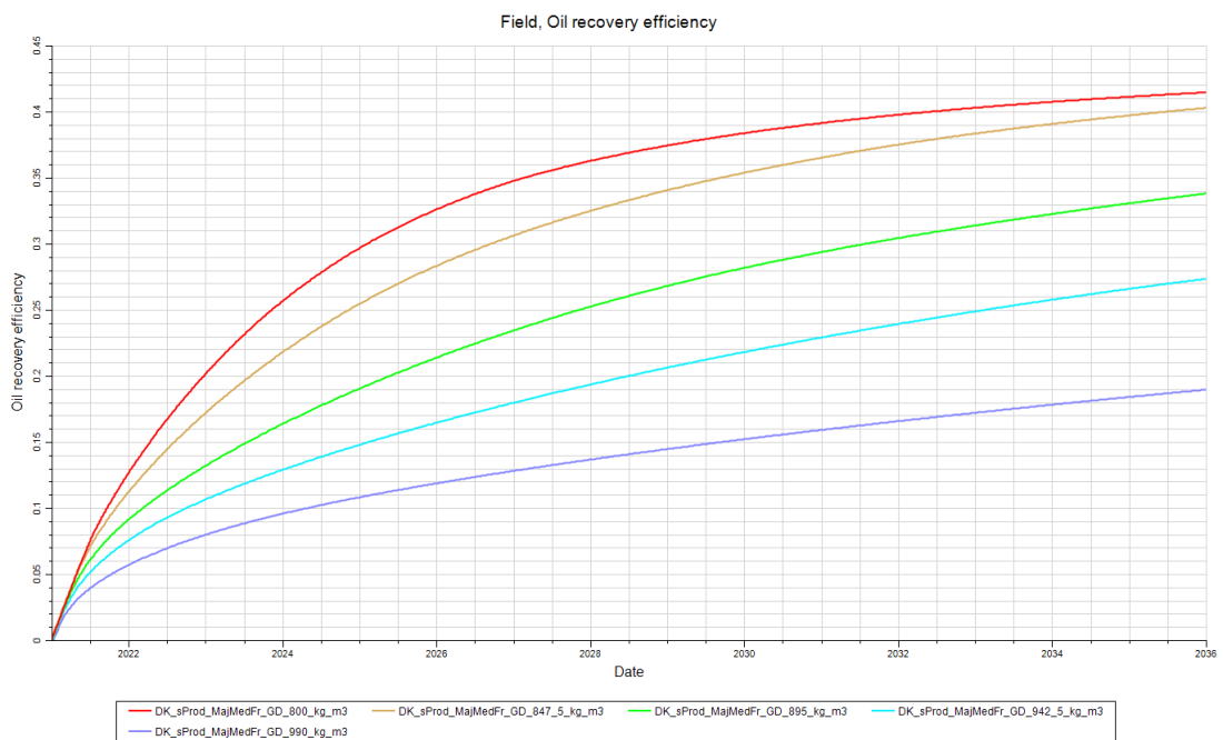
Figure 58: Gas injection viscosity sensitivity utilizing major and medium fractures
