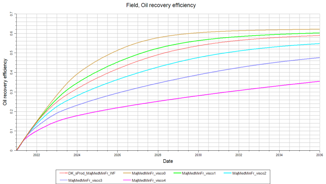
Figure 84: 3D waterflooding viscosity sensitivity utilizing major, medium, and minor fractures
