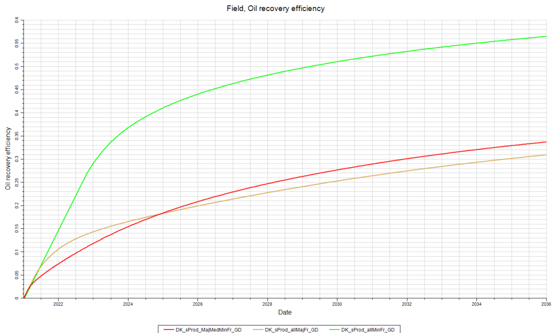
Figure 49: Comparison in recovery efficiency in case of all major and all minor fractures
