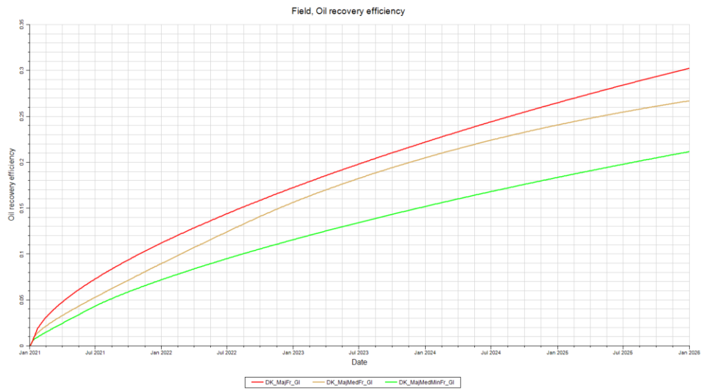
Figure 33: The recovery efficiency for secondary production gas injection in the extended vertical slice
