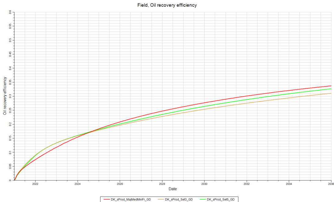
Figure 48: Fracture distribution sensitivity for gas injection case
