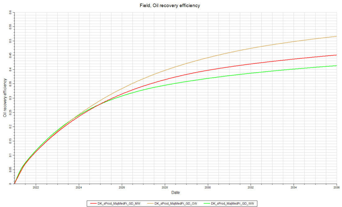
Figure 55: Wettability sensitivity runs with major and medium fractures included for gas injection
