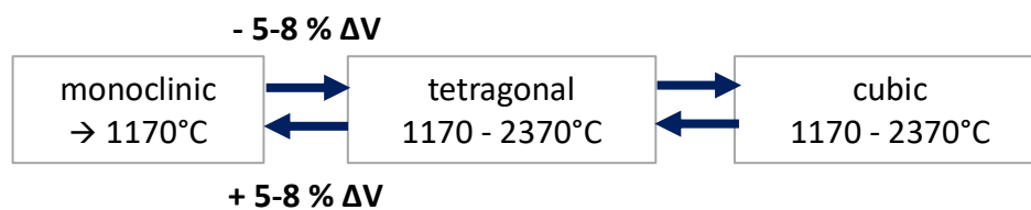
Fig. 5: Schematic phase transformation of zirconia
