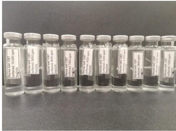
Figure 4-3 Alkaline solution (softened brine) at different concentrations
