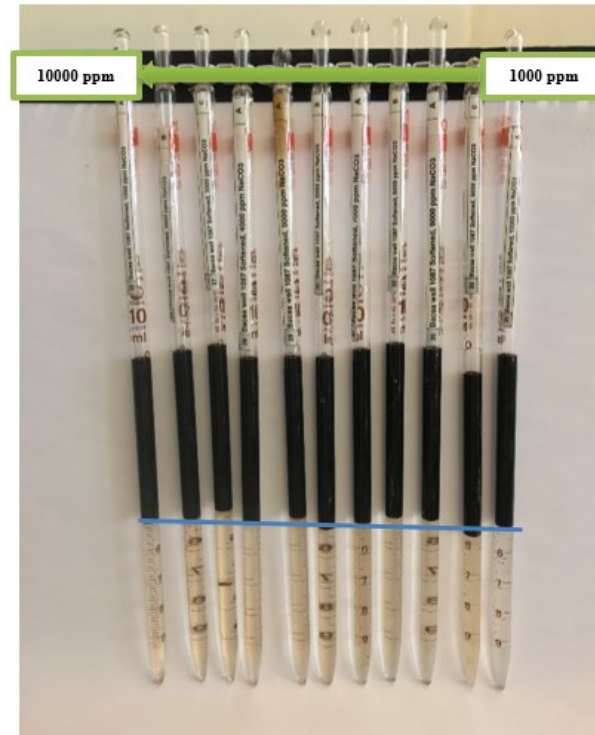
Figure 5-29 Phase experiments with Alkaline solution at (1000-10000) with 1000 step, Blue lines: oil/brine interface.
