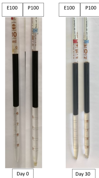
Figure 5-28 Phase experiments with 0.1 wt% of nanofluid P100 & E100, Blue lines: oil/brine interface
