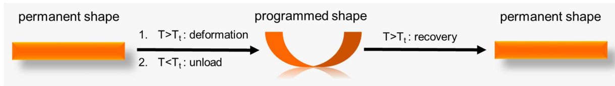
Figure 20: Schematic illustration of a shape changing process in SMPs
