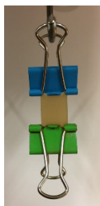
Figure S5 – Photograph of a typical repaired elastomer sample fixed between two clamps used for stress-rupture tests. To the lower clamp the respective weights with different masses were attached.
