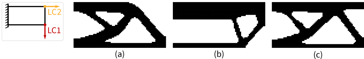
Figure 5.7.: Optimal design of the cantilever beam determined with the standard topology optimization method Q-Iso . (a) Optimized for Loadcase A (LC1), (b) Optimized for Loadcase C (LC2), (c) Optimized for both loadcases ( Loadcase AC ).
