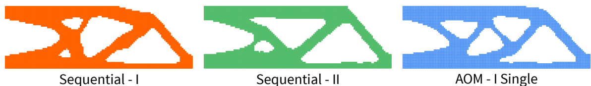
Figure 4.21.: Comparison of sequential and simultaneous optimization for a cantilever beam with dimensions 60 mm x 20 mm for Loadcase A ( m_{\text{size}} = 0.5 mm, r_{\text{min}} = 3 mm, ER = 0.01 )
