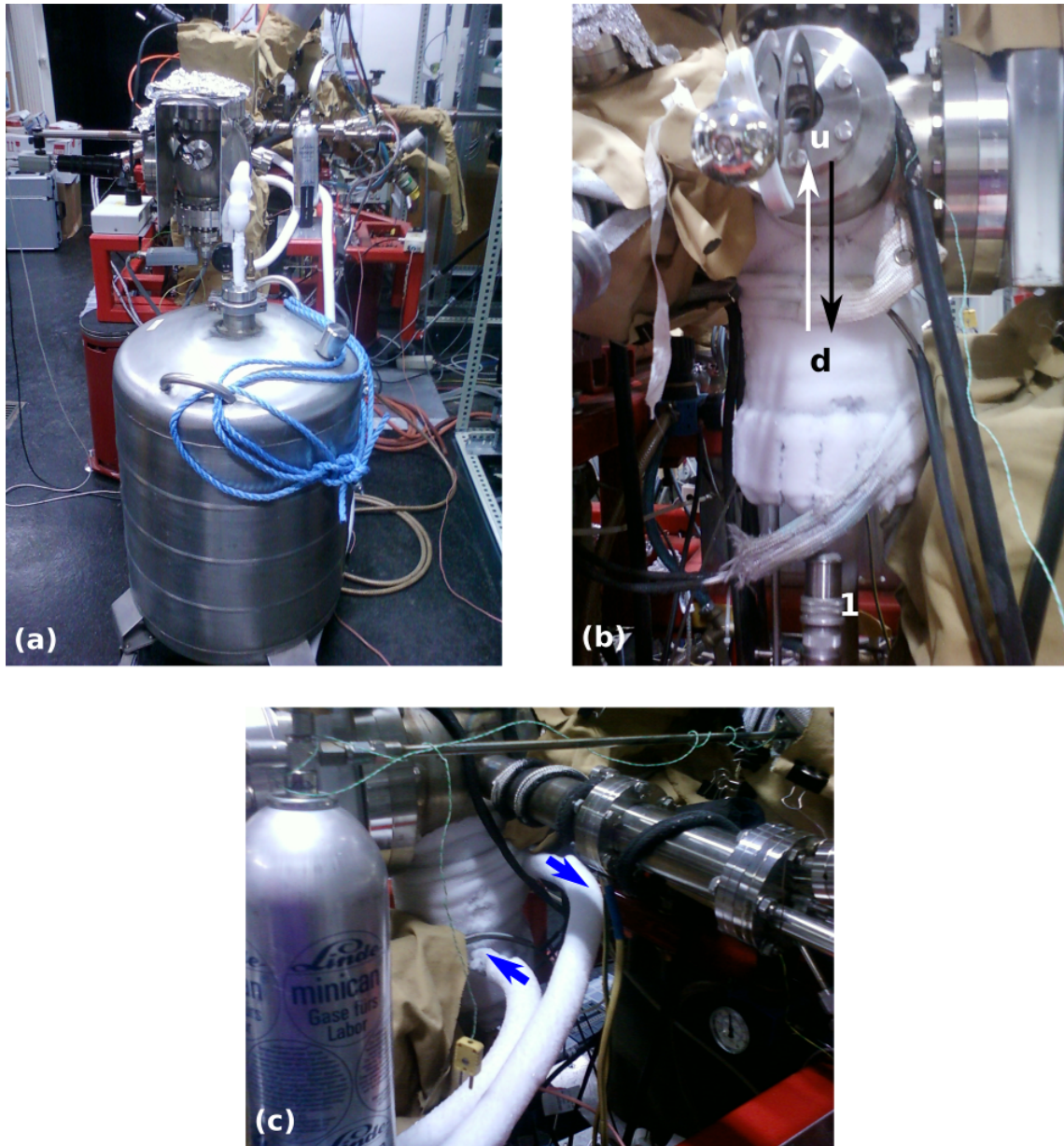
Figure 3.6: Growth experiments with passive cooling by liquid nitrogen. (a) Dewar filled with liquid nitrogen in front of the UHV system. (b) Front view of the growth chamber with its lower part cooled from outside (1...manipulator of the heater; u and d indicate the approximate heater upper position during annealing & thin-film growth and lower position during sample transfer & passive cooling; white and black arrows indicate the vertical moving direction of the heater inside the growth chamber). (c) Rear view of the passive cooling system (blue arrows indicate the flow direction of the liquid nitrogen).
