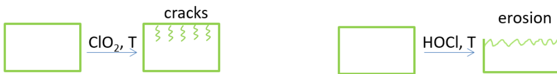
Fig. 5.24: Schematic illustration of the PE surface aging in contact with ClO 2 and HOCl disinfected aqueous solutions.
