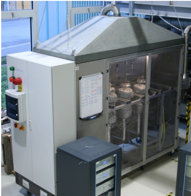
Figure 4-1: Methanation laboratory scale test plant at VTiU
