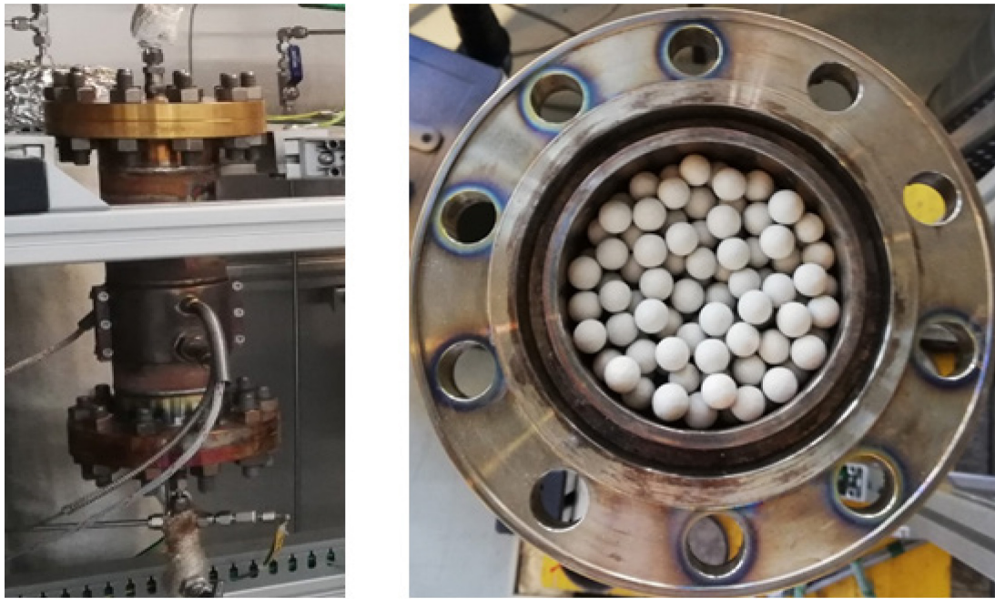
Figure 4-3: Fixed-bed reactor without insulation (left) and with opened flange (right)
