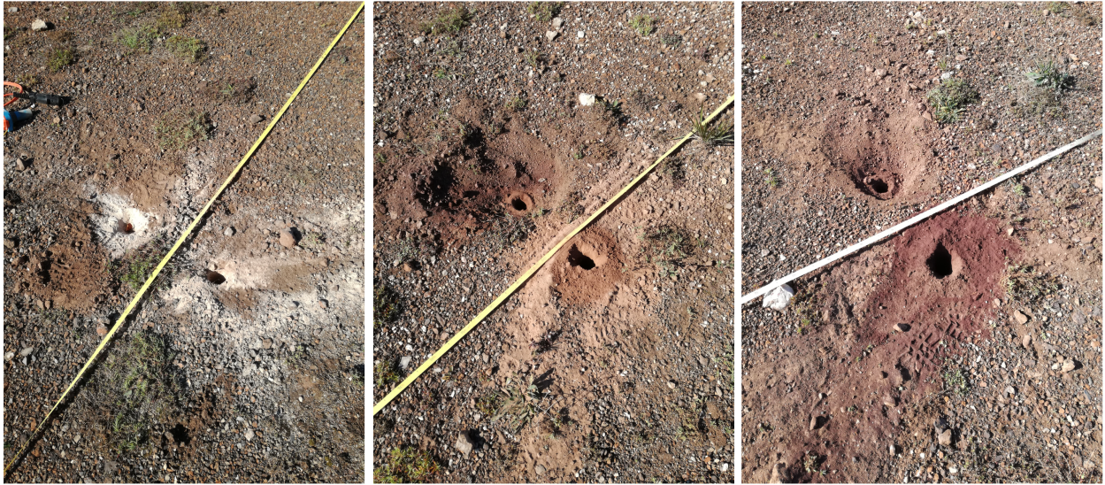
Figure 4.3.2: Borehole cuttings from the boreholes drilled for the explosive sources showing three different coloured lithologies ranging from white, bright grey (left) to reddish brown, ochre (middle) to dark reddish brown (right)
