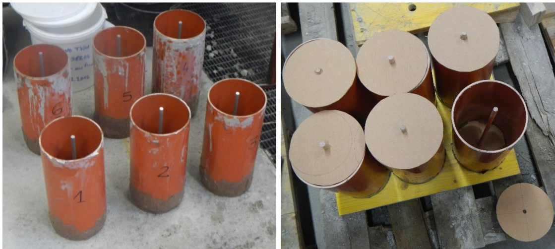
Figure 191: Confinements for casting the mortar cylinders.
