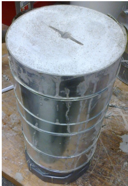
Figure 233: An earlier cylinder-wrapping solution with an aluminium sheet bent around the cylinder and held together with a tightened steel wire (blast test 9).
