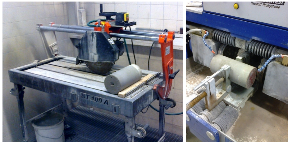
Figure 194: Equipment used for transverse cutting of the cylinders.
