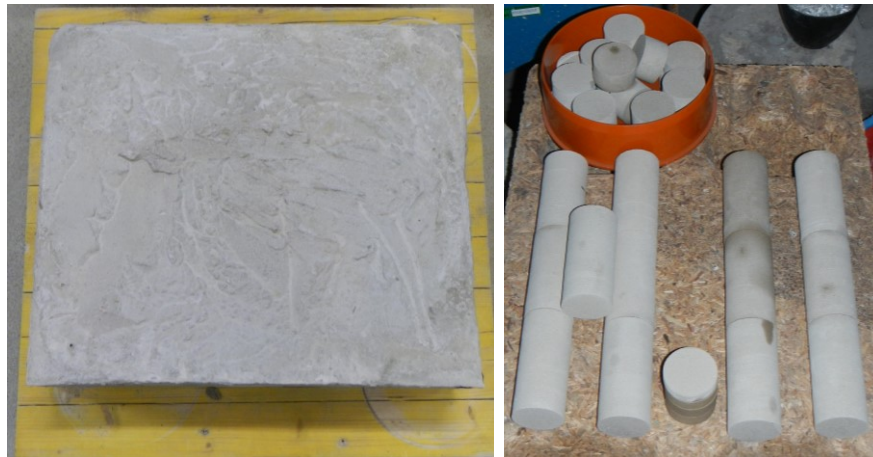
Figure 196: Block for producing material-testing samples of mortar (left) and the samples after core-drilling (right).
