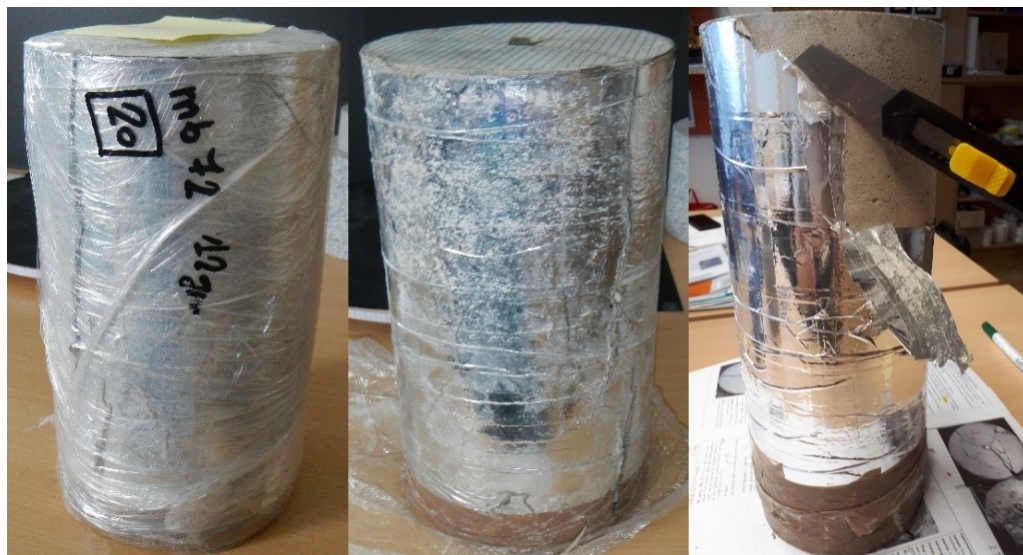
Figure 32: Removal of protective foils from blast cylinder mb-72, m12(20).
