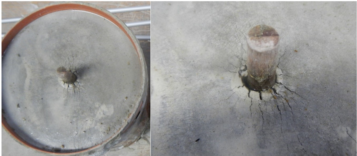
Figure 193: Radial drying-induced cracking around the sticks at the end-face surfaces.
