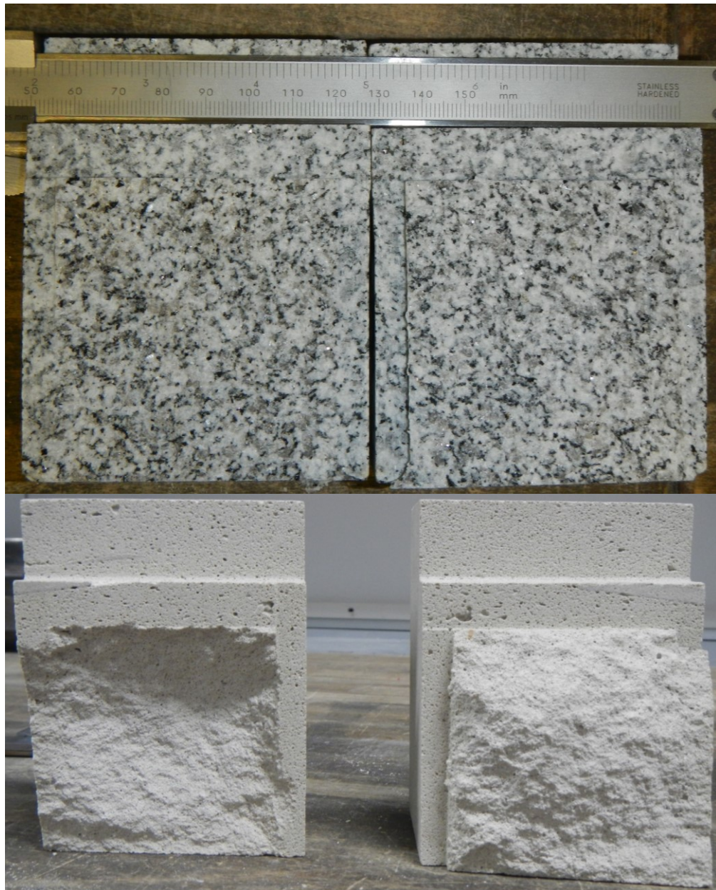
Figure 208: Typical resulting fracture surfaces from WSTs on the granite (top) and the mortar (bottom).
