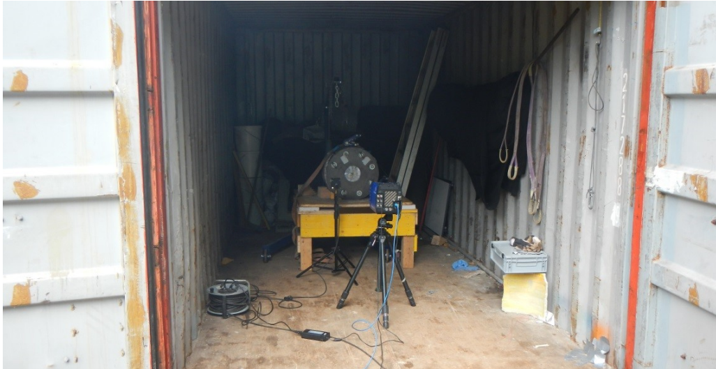
Figure 231: Common blast set-up with the blast chamber and the HSI camera inside an enclosed transport container.
