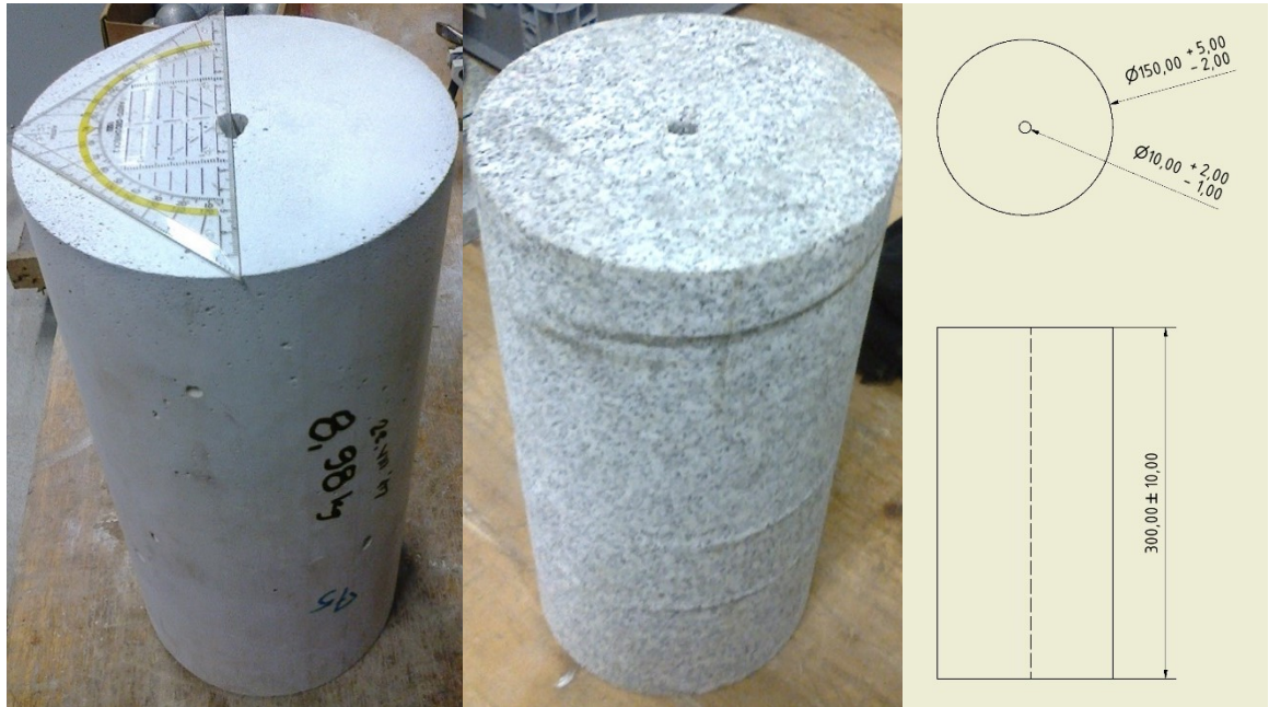
Figure 17: Blast cylinders before blasting.
