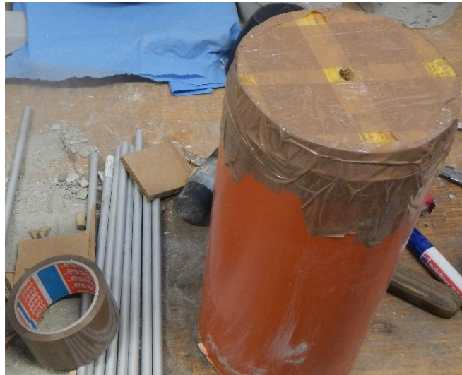
Figure 192: Sealed mortar-casting confinement.
