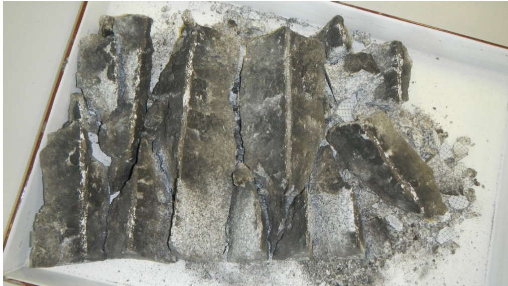
Figure 79: Blasted cylinder taken apart and prepared for sieving (g12(25)).
