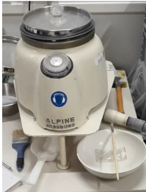
Figure 245: Apparatus for air-jet screening (laboratory of the Chair of Mineral Processing, IZR, MUL).
