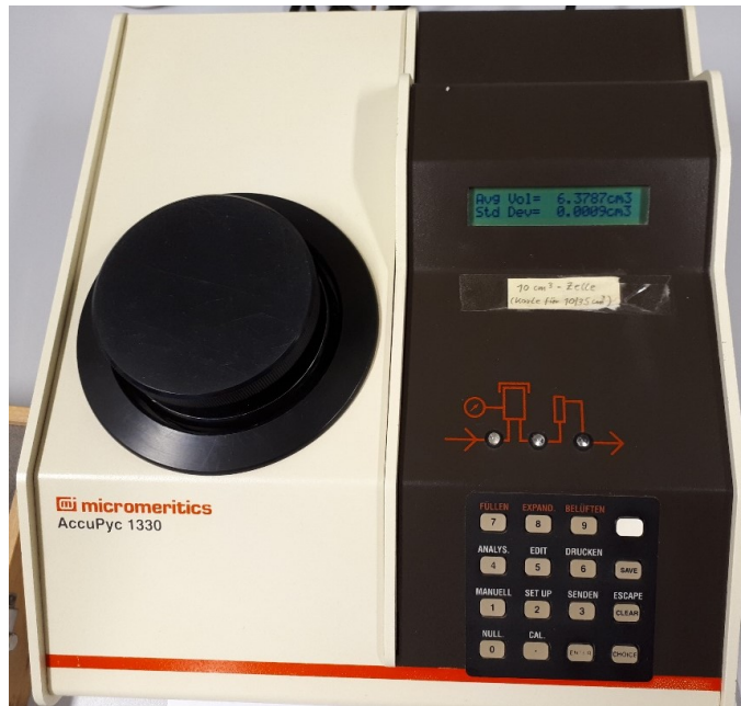
Figure 201: Gas pycnometer Micromeritics AccuPyc 1330 (laboratory of the Chair of Mineral Processing, IZR, MUL).
