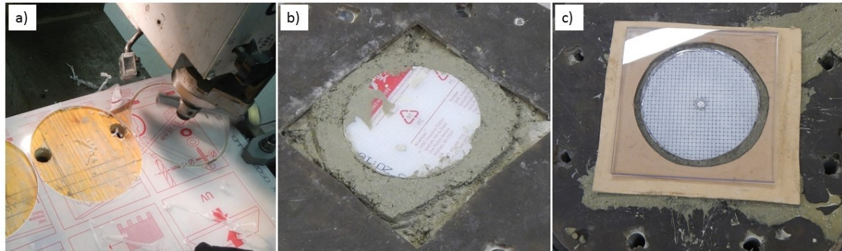
Figure 234: Replaceable polycarbonate disk: a) being manufactured; b) placed directly on a blast cylinder; c) covered with the protective window prior to a blast test.
