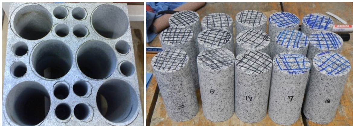
Figure 199: Original granite block (left) and cylindrical material-testing samples (right).
