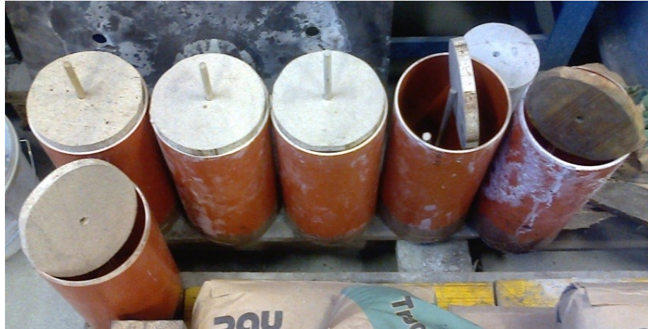
Figure 18: Casting moulds for the mortar blast cylinders.
