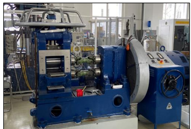
Fig. 5. Rolling mill system at the MF (300 kN).
