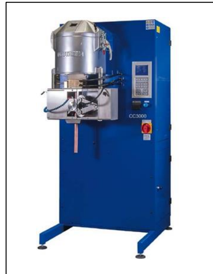
Fig. 3. Continuous casting aggregate at the NFM [10].
