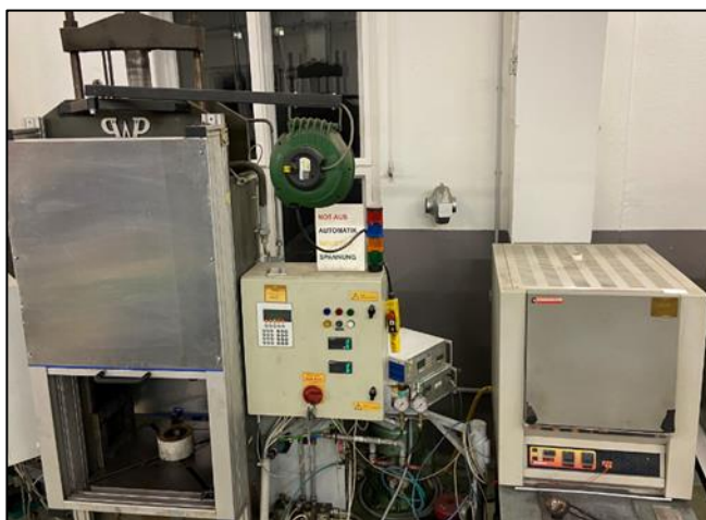
Fig. 4. Hydraulic press with control unit (left), furnace (right).
