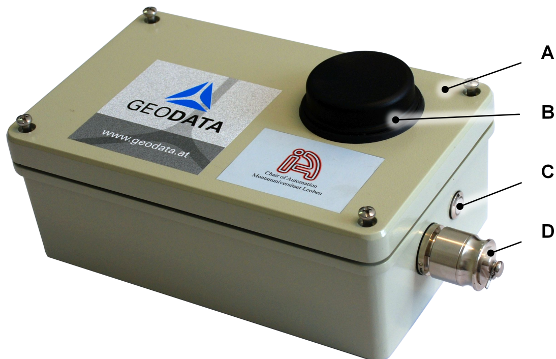
Fig. 4.3 Wireless Measurement Box: A) robust aluminium case B) IP67 antenna for 800MHz to 2.5GHz C) LED-button for triggering predefined actions. D) IP67 Ethernet connector
