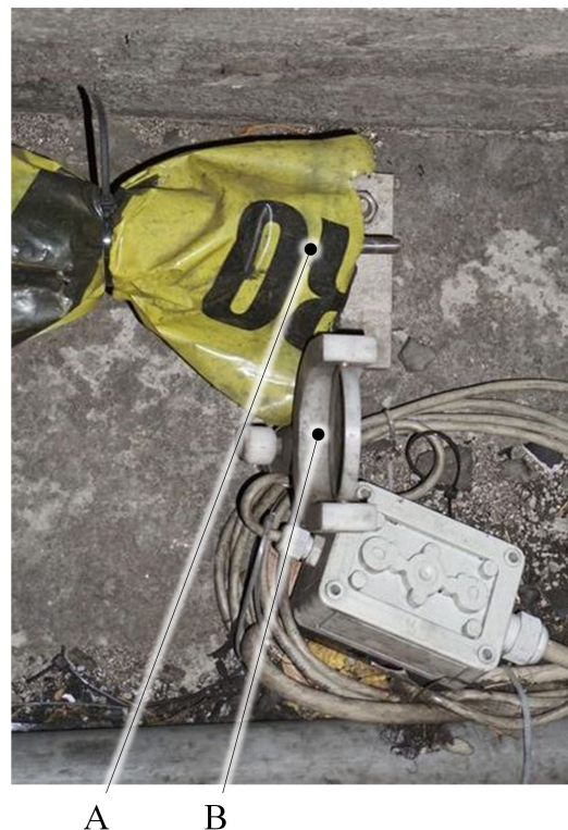
Fig. 3.22 Photograph of the end of the inclinometer chain (A) together with a retro-reflector (B) for the total station measurements. © Geodata GmbH.
