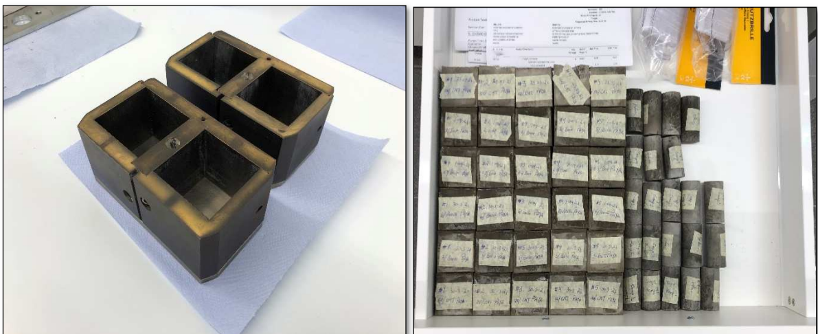
Figure 22 - left) Cube Molds right) Prepared Cubic and Cylindrical Samples
