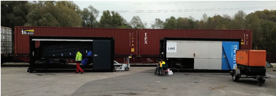
Figure 6.7: First field test constellation: Two plant units were arranged in a predefined relative position in an industrial environment, not yet connected through a conveyor belt.
