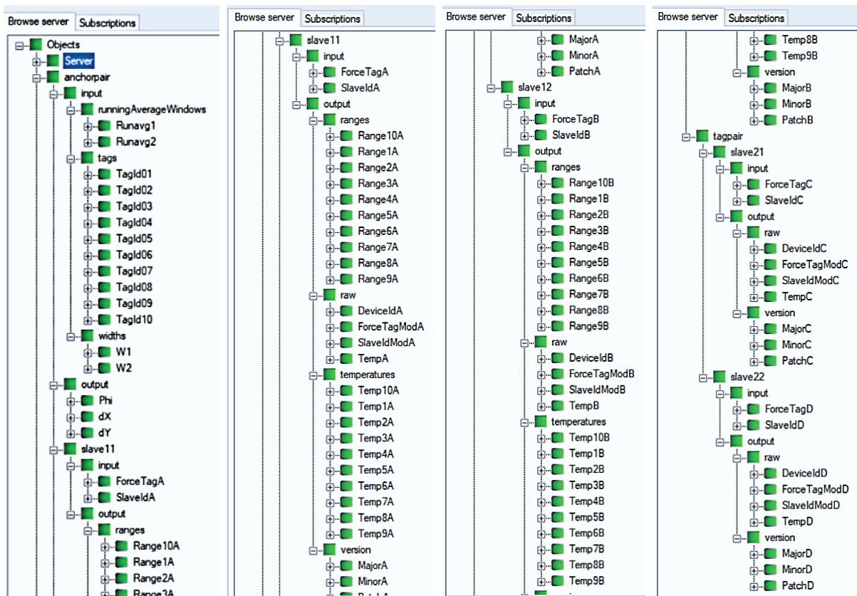
Figure A.1: The whole OPC-UA variable tree is composed of object nodes. The first one is the Server object node, while the leaf nodes are the variable nodes.
