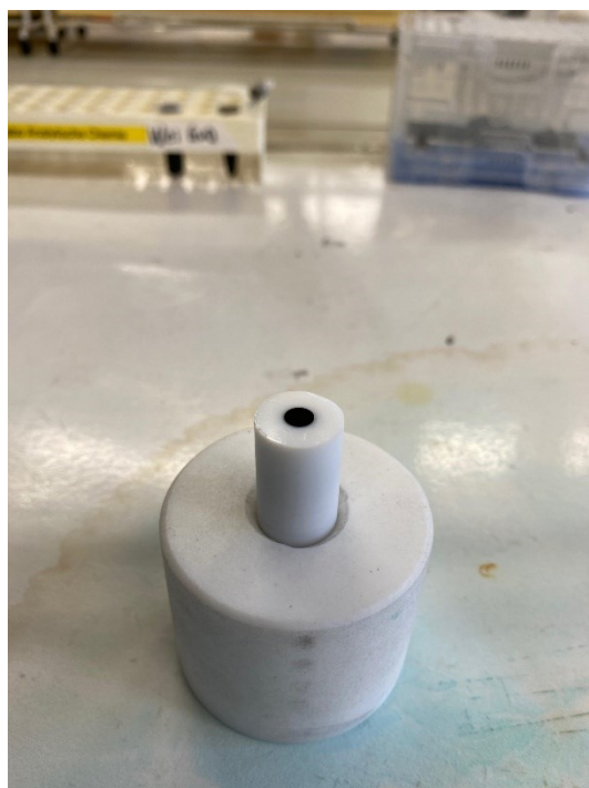
Figure 33: Catalyst ink covered rotating disc electrode
