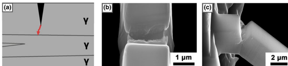
Figure 6: For specimen (L)_C1 (a) a sketch of the observed crack path through \gamma lamellae with (b) the corresponding fractured surface and (c) a side view showing the crack path are displayed. Since the type (L) cantilevers were located at the same position within the \alpha_2/\gamma colony, corresponding lamellae were tested and only one representative sketch and fractured surface are displayed.
