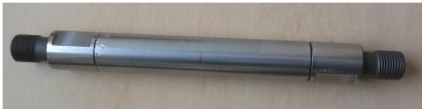
Figure 8: Downhole Dynamometer Sensor
