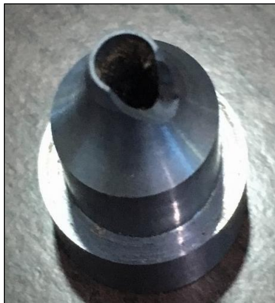
Figure 13: Damaged nozzle due to cavitation.
