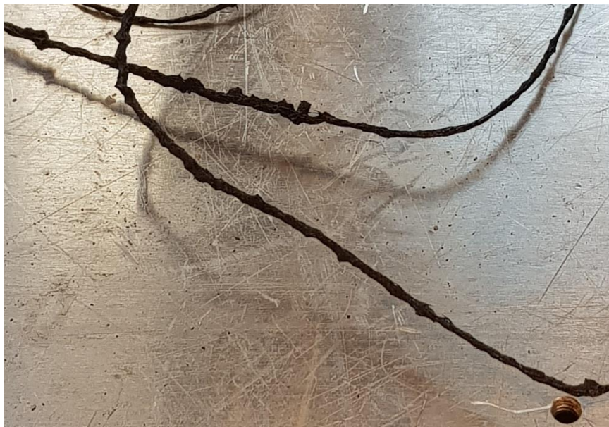
Figure 4.16: Melt fracture phenomenon in lab experiment for PA66GF30
