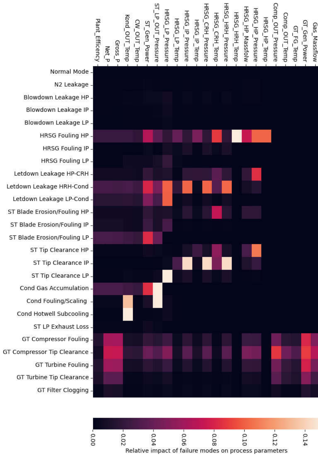
Figure Appendix 2: Heatmap for the relative impact (scale up to 15%) of every failure mode on the process parameters
