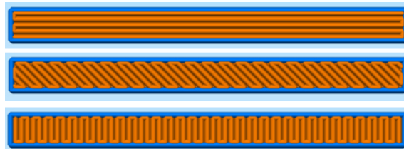
Figure 1. Fill pattern of perimeters (blue) and infills (orange) of one layer for specimens of each of the infill orientations, from top to bottom: 0°, ±45° and 90°.
