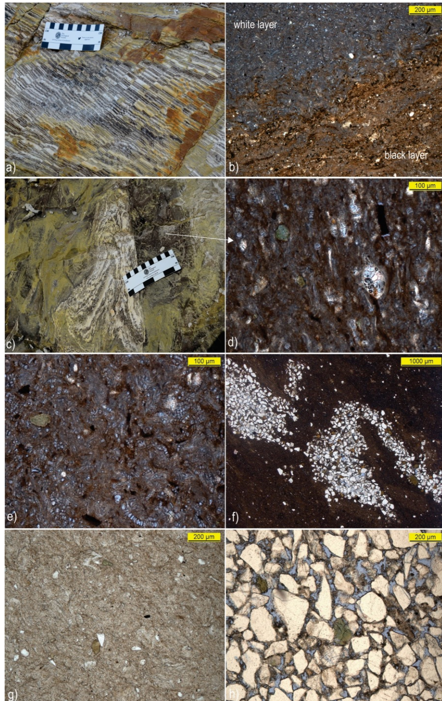
Figure 4.16. Selected samples and thin-section photographs from Sibiciu de Sus quarry. a, b-highly faulted alternation of white and black diatomite [a], the white layers contain significantly less organic matter compared with the black ones [b] (sample S17); c, d, e-impure diatomite highly deformed and faulted, covered with sulphides containing abundant organic matter [c], volcanic vacuolar glass [d] (sample S1) and intact diatoms frustules [e] (sample S10); f-pure diatomite with diatom mass and rare organic matter with few sandstone deformations present (sample S19); g- chert with few detrital grains: angular quartz, feldspars and glauconite (sample S21). h – quartz-rich sandstone containing angular quartz and glauconite with siliceous cement (sample S15).
