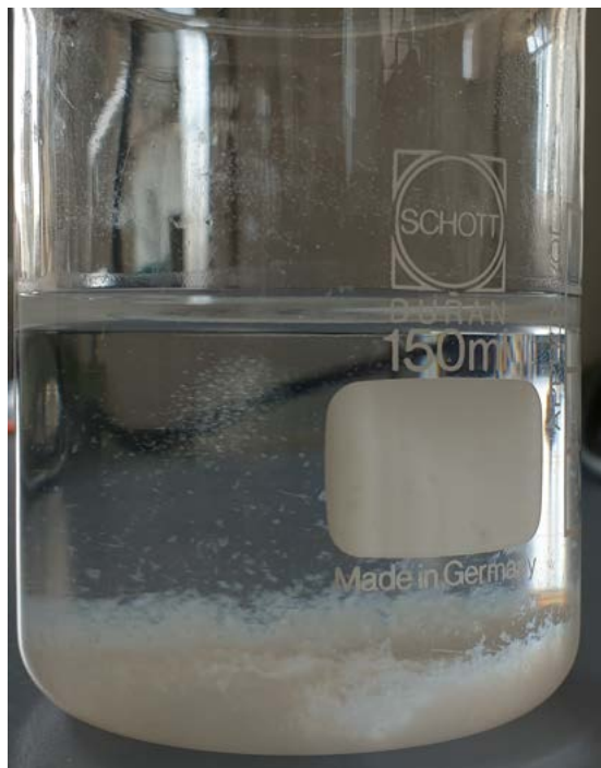
FIGURE 5.3: Precipitation in the formation brine/alkali solution
