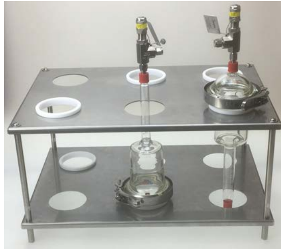
FIGURE 4.15: Amott cell for imbibition (left) and drainage (right) (Pan-Terra 2020)
