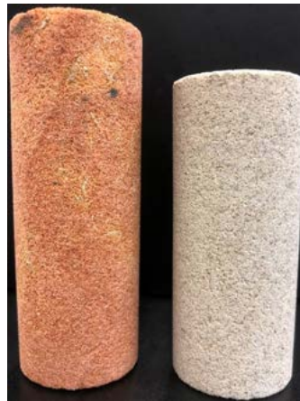
FIGURE 4.1: Core plugs (From left to right) Keuper - Berea
