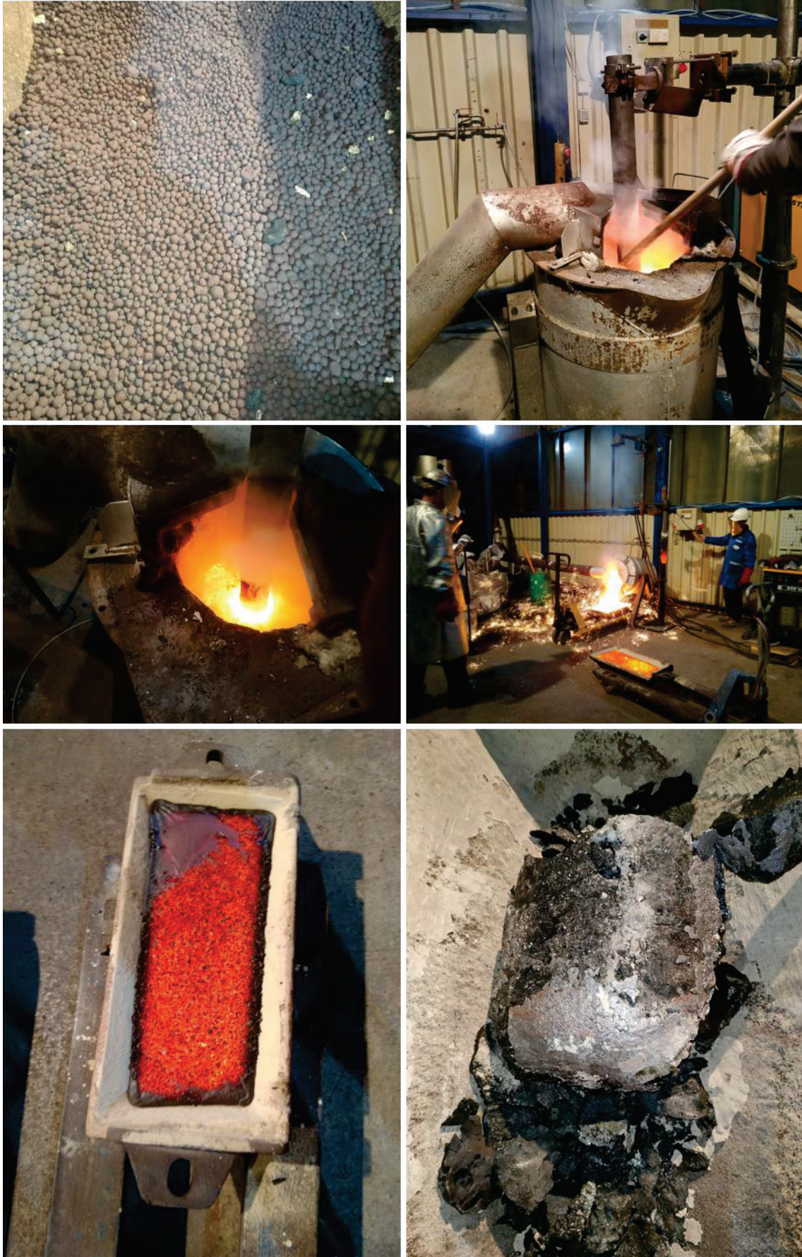
Appendix 32: Reduction trials with jarosite from zinc production. Upper left: calcine. Upper right and middle left: reduction in the electric furnace. Middle left: tapping. bottom left: slag. bottom right: slag and alloy.
