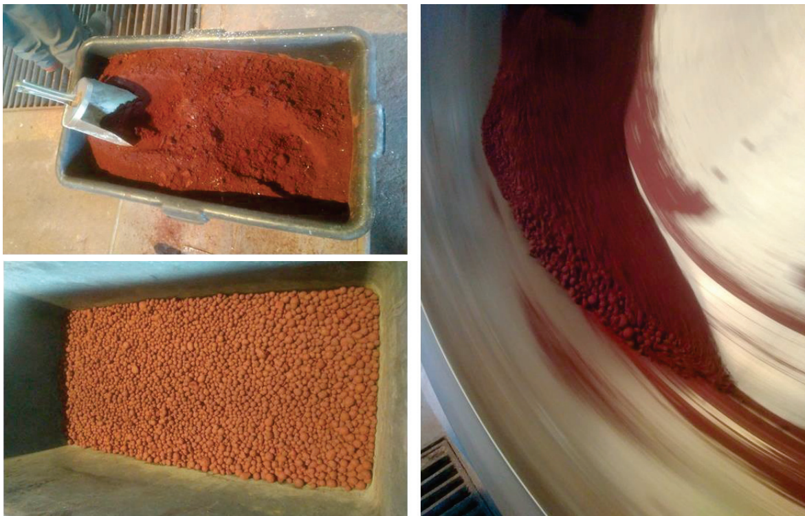
Figure 66: Upper left: jarosite from platinum production mixed with calcium hydroxide ready for pelletizing (first trial). Right: Agglomeration process. The pelletizing disc is the same as in Figure 58. Lower left: finished pellets of about 0.5-1.7 cm in diameter.
