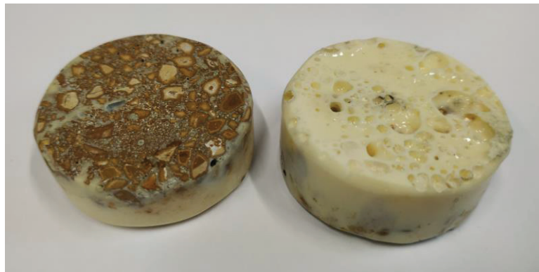
Figure 9: Example of two jarosite sections using a fast hardening and high viscosity epoxy resin. The sections are 4 cm in diameter.
