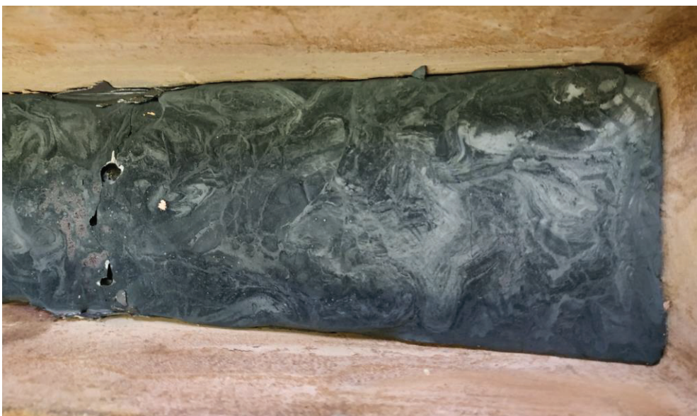
Figure 60: Synthetic pre-slag of fayalite composition. The mould is about 15 cm wide.
