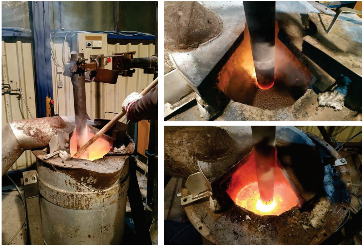
Figure 61: Left: Electric furnace used for reducing the jarosite calcine. Upper right: Calcine is fed but not yet completely molten. White smoke indicates evaporating zinc. Lower right: The whole load is molten. White smoke is nearly gone.
