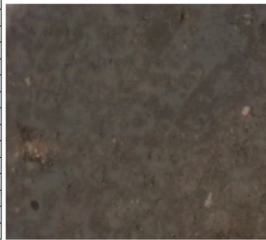
Appendix 10: RAMAN measurement of a jarosite particle in a jarosite residue from zinc production.
