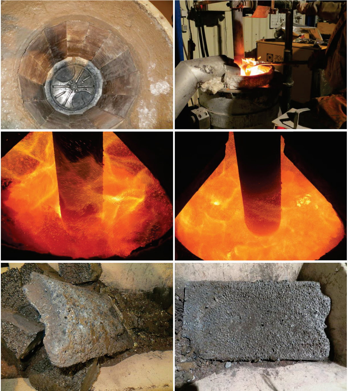
Appendix 49: Reduction trials with jarosite from platinum production. Upper left: Electric furnace prepared for trials. Upper right: sampling during reduction trial. Middle: liquid slag. Bottom: slag and alloy after tapping.
