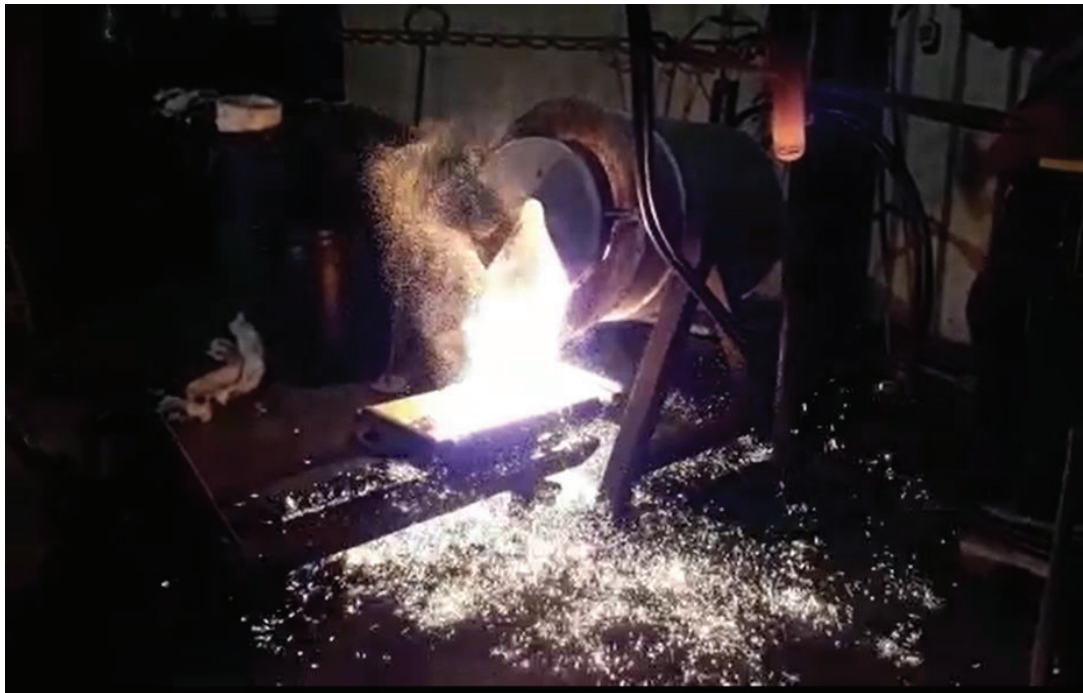
Figure 67: Tapping of the jarosite from platinum production after reduction. The sparks on the floor are caused by oxidation of metallic iron and the rising burning carbon powder.
