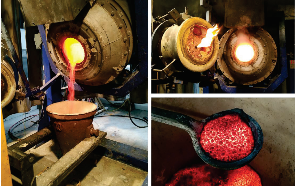
Figure 59: Left: Tapping of calcine from the TBRC. Upper right: opened cap of the TBRC. Note the flame of the gas burner. Lower right: freshly calcined, still-glowing jarosite pellets.
