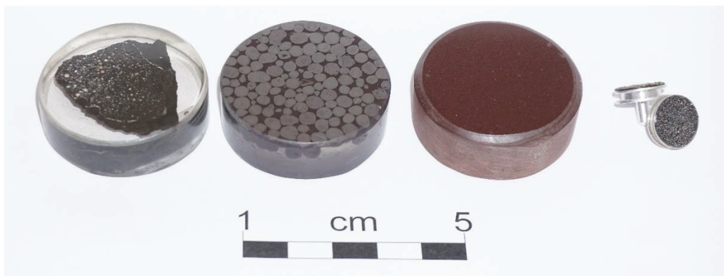
Figure 40: Different samples prepared for investigations using a scanning electron microscope. The three samples to the left are embedded in epoxy and polished. The diameter is 4 cm each. From left to right: final slag, roasted pellets (calcine) and original residue. The sample on the right is a strewn slide on double-faced adhesive tape.
