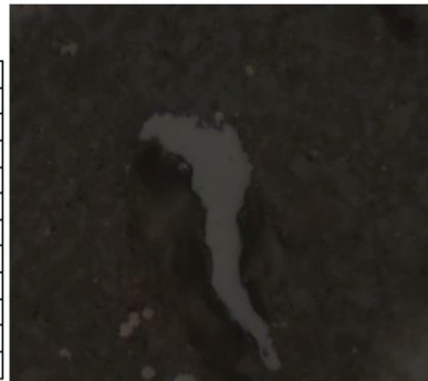
Appendix 11: RAMAN measurement of a sphalerite in a jarosite residue from zinc production.
