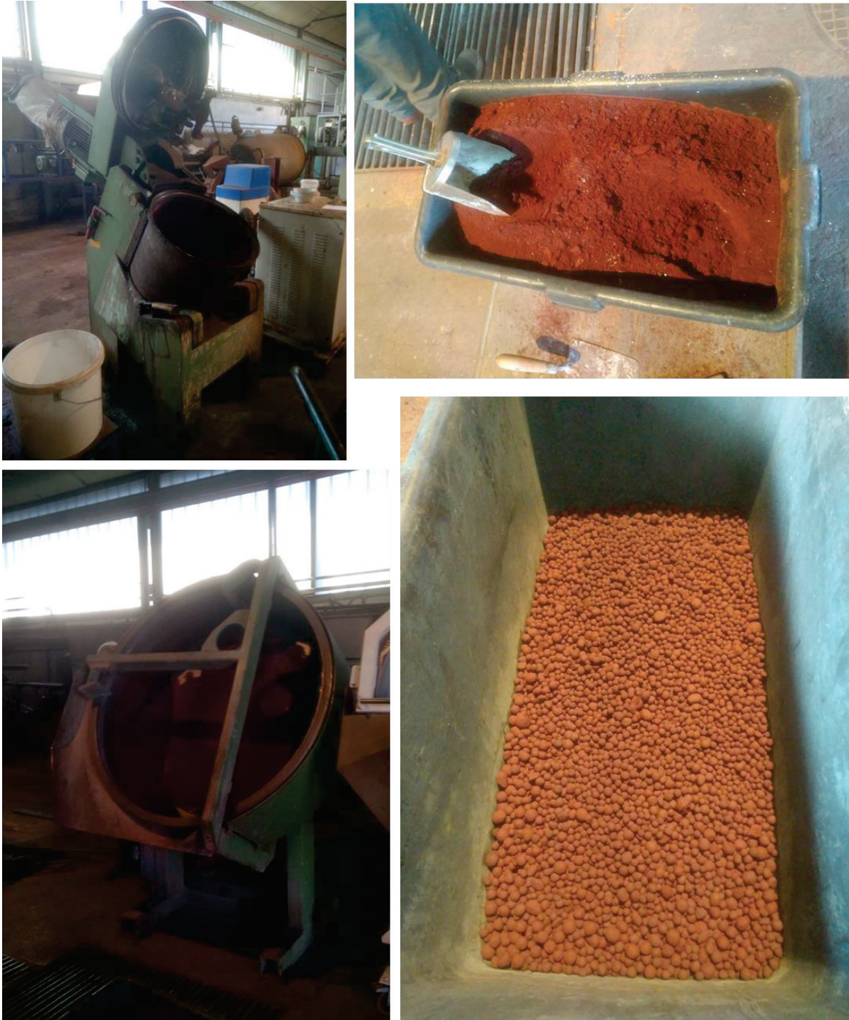
Appendix 47: Preparation of jarosite from platinum production for pyrometallurgical treatment. Upper left: mixer. Upper right: Jarosite from platinum production mixed with calcium hydroxide. Bottom left: pelletizing disc. Bottom right: pellets ready for calcination.
