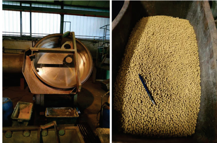
Figure 58: A disc pelletizer (left) was used to agglomerate the jarosite. The right picture shows the jarosite pellets.
