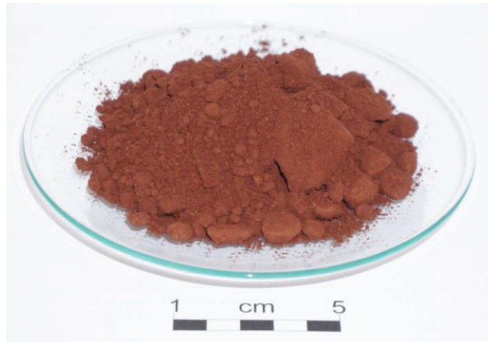
Figure 5: Dried jarosite residue from platinum production.
