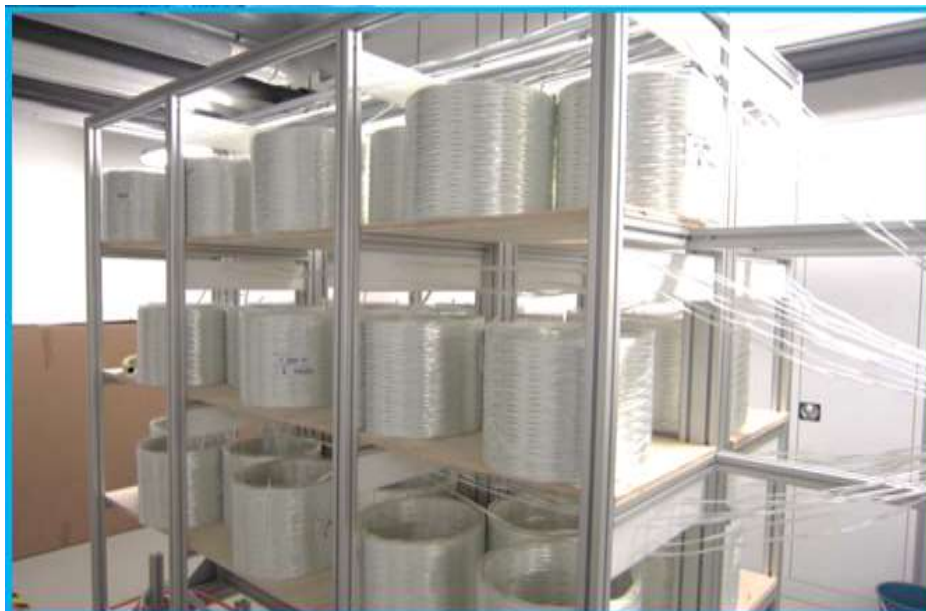
Fig. 6. Spool box equipped with glass fibre tow spools.
