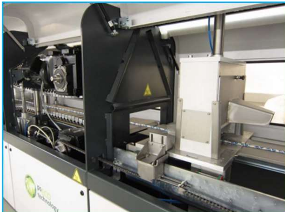
Fig. 12. Pulling machine equipped with a cut-off station (Source: LVV, Montanuniversität Leoben).
