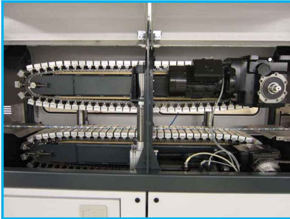
Fig. 11. Pulling machine equipped with a cut-off station (Source: LVV, Montanuniversität Leoben).
