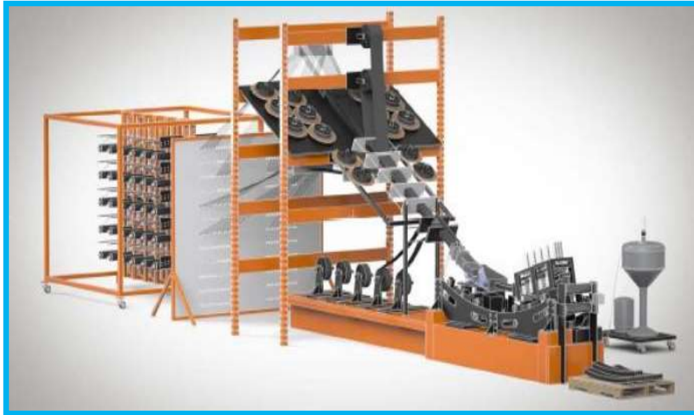
Fig. 14. Radius pultrusion process (Figure Source [19])
