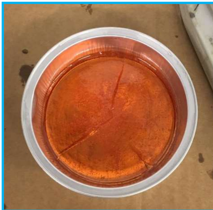
Fig.39. Epoxy resin derived from an unmodified liquid diglycidyl ether of Bisphenol A (DGEBA resin) in a mixture with an Anhydride Curing Agent and an Accelerator like DMP-30 (2,4,6-tris(dimethylaminomethyl) phenol).
