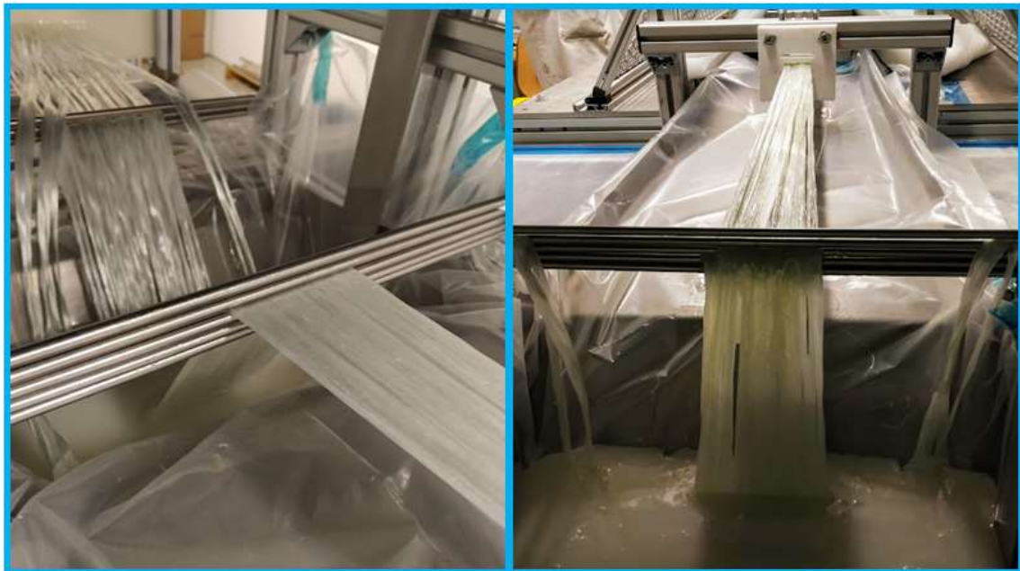
Fig. 7. An open dip-type resin bath.
