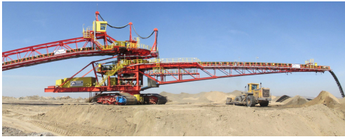
(a) Mobile Tripper Spreader, part of the material-supplying mobile tripper car can be seen on the left [40] (typical)
