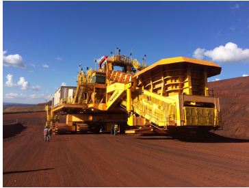
(a) Mobile Primary Crushing System during relocation [23]
