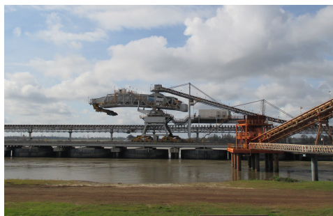
(a) Slew/Luff/Shuttle Ship Loader
