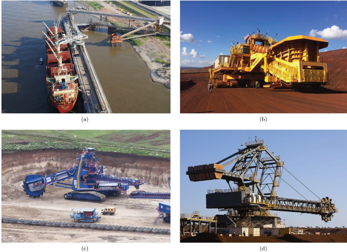
Fig. 4: Examples of four systems that are currently being monitored using the described approach: a) ship loader, b) mobile sizing rig, c) bucket-wheel excavator, d) bucket-wheel reclaimer. The sensor channels of these systems are monitored with a sampling interval of 1s. (Sources: (a) – http://www.flickrriver.com/photos/impalaterminals_images/17557941415/ , retrieved on 2016-02-08; (b), (c), (d) – Courtesy of Sandvik.)
