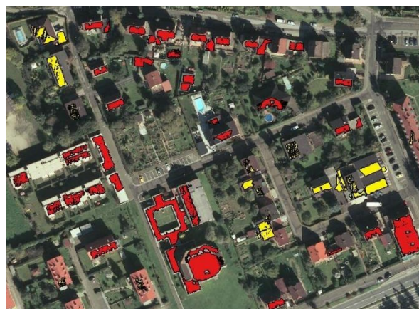
Figure 4-21: Example of identified rooftop potentials. “Very good” rooftop areas are marked in red – “Good” rooftops areas are marked in yellow
