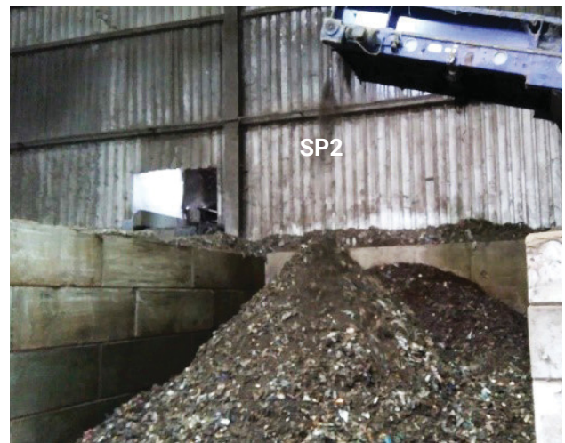
FIGURE 6: Input material after a shredder and an overbelt magnet, SP1 (left) and fines from the first screen 60 mm, SP2 (right).
