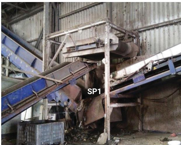
FIGURE 6: Input material after a shredder and an overbelt magnet, SP1 (left) and fines from the first screen 60 mm, SP2 (right).
