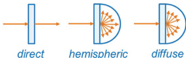
Figure 3. Measurement of direct, hemispheric and diffuse transmittance.
