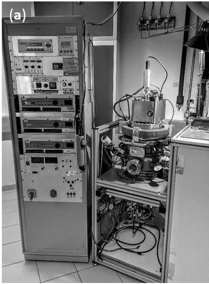
Fig. 2.5 (a) Custom-built laboratory scale dc magnetron sputter device. (b) View inside the operating deposition chamber.
