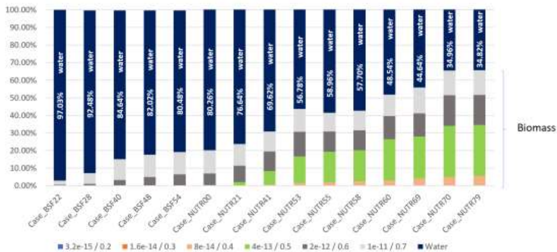
Figure 15: Illustration of the change in pore space composition. Dark blue colored blocks refer to water, the other blocks represent the biomass with varying permeability and porosity.
