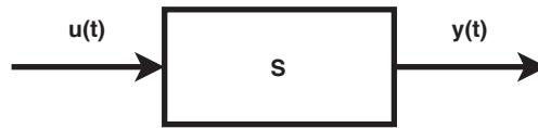
Figure 1.1: Block diagram model of a system with an input u(t) and an output y(t) .
