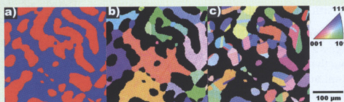
Fig. 4: a) phase map (blue ferrite, red austenite), b) IPF of the ferrite phase and c) IPF of the austenite phase of the duplex steel
