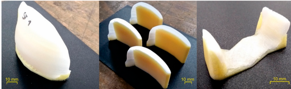
Figure 9. Benchmark “implants” printed with the optimized printing parameters (“PMMA final values” in Table 2).
