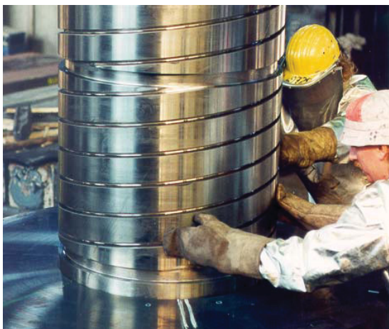
Figure 1: Shrink-fitting of a liner holder
