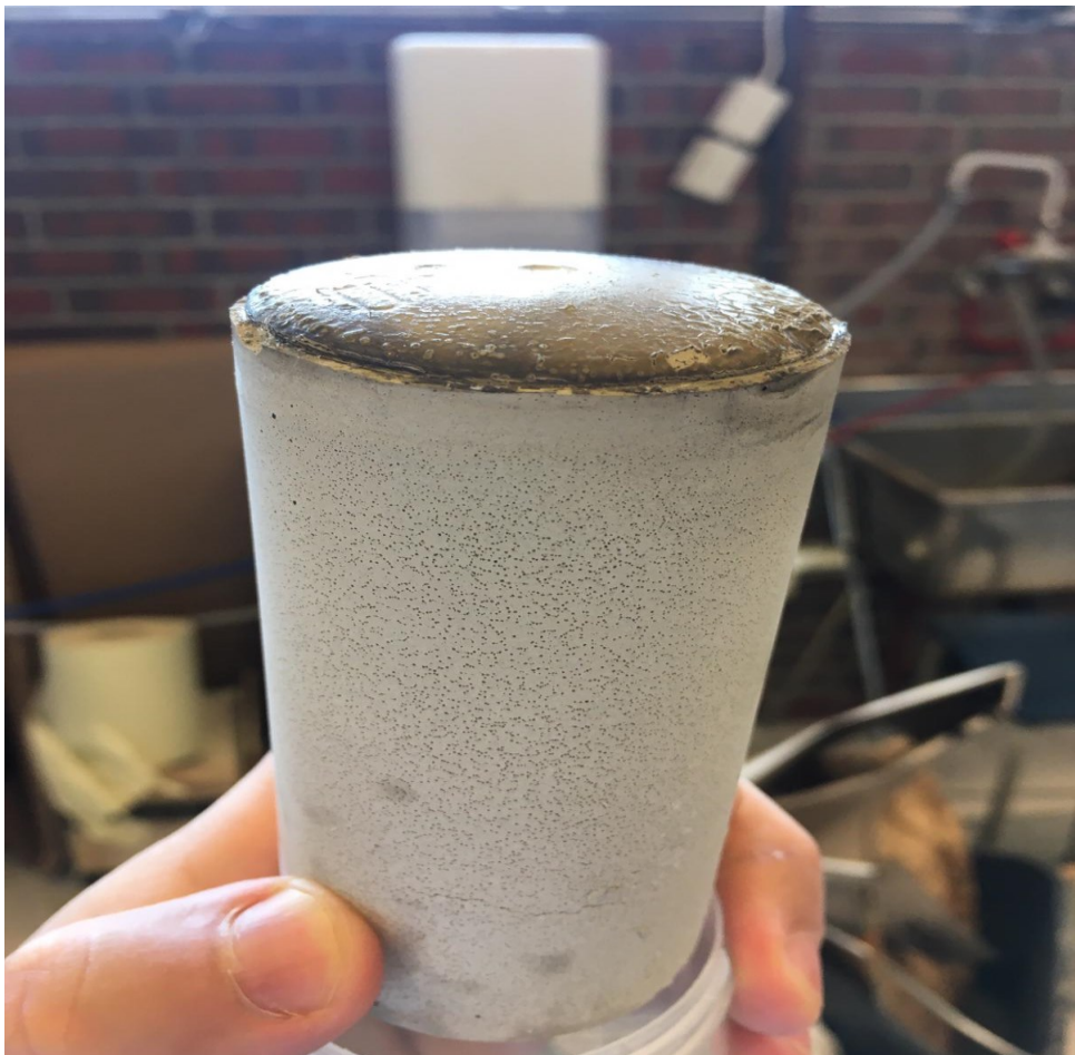
Figure 6-9 The Consequences of Gas Bubbles on Curing
