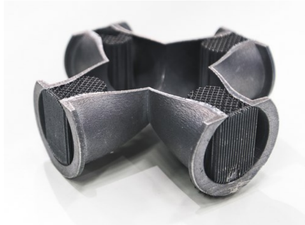
Figure 50: Support structure attached to an AM part (3D Hubs/Redwood 2018)
