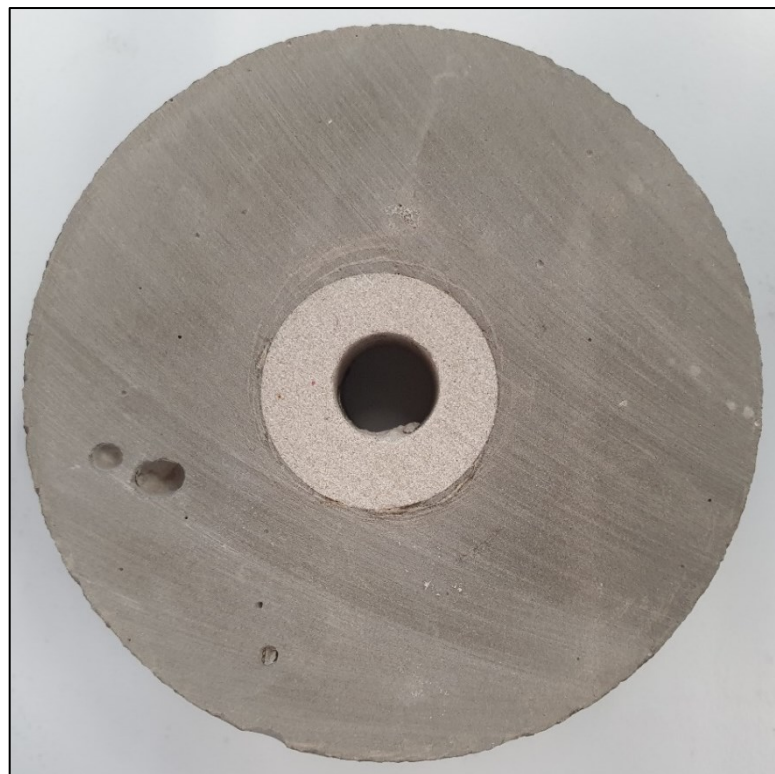
Figure 56: Cut and dried disk of the 17 ppg cement after extraction from the autoclave.
