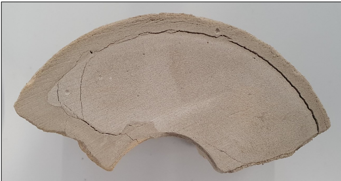
Figure 41: Cut and dried piece from one of the segments of the 11.5 ppg cement after carbon dioxide exposure.
