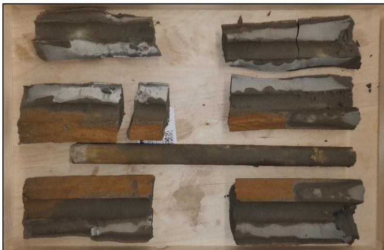
Figure 40: Photograph of the cement and sandstone after extracting it from the autoclave.
