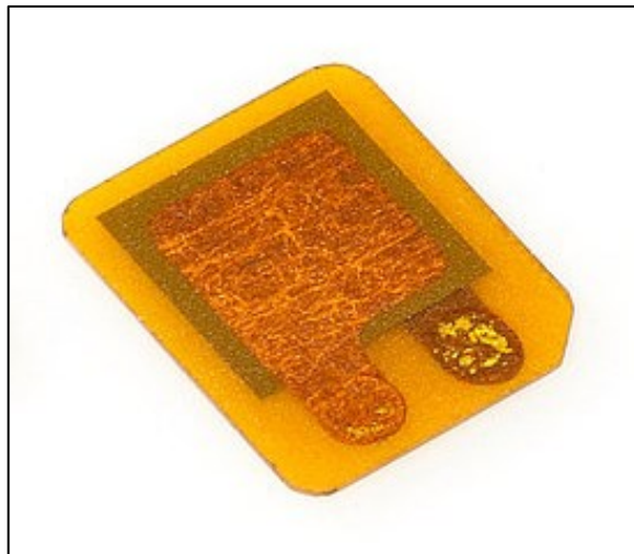
Figure 6: The piezoelectric element utilized for the cement analysis in this thesis.
