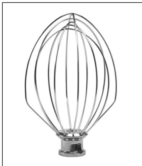
Figure 13: Stirrer utilized to mix the cement slurry in the batch mixer.
