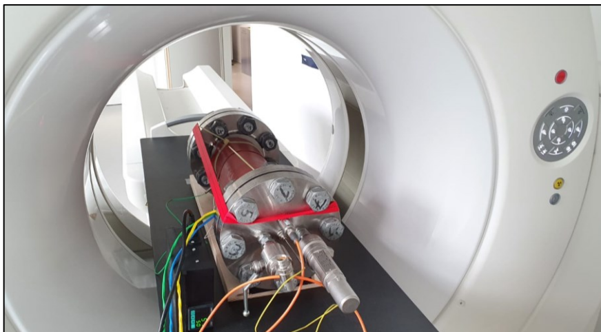
Figure 35: Photograph of the autoclave inside the CT-scanner.
