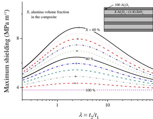
Figure 4. Influence of the AZ-composite chemistry on the maximum shielding of the outer A-layer
