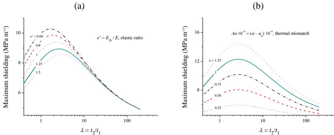
Figure 5. Influence of the Young's modulus  $E$  and of the coefficient of thermal expansion  $\alpha$  on the maximum shielding.
