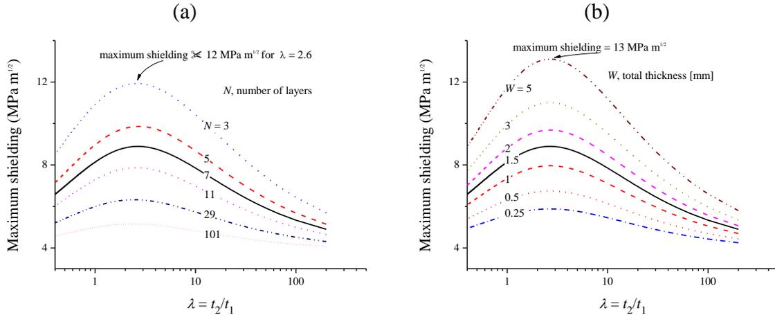
Figure 3. Influence of architecture on shielding. A)  $N$ , Number of layers, B)  $W$ , Total thickness.
