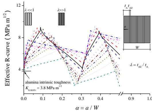
Figure 1. Influence of the thickness ratio  $\lambda = t_{AZ}/t_A$  on the effective R-curve. The situation  $W = 1.5$  mm and  $N = 7$  layers has been chosen to present the results.
