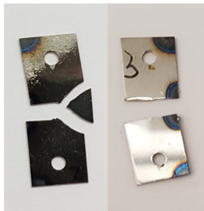
Figure 5.21: Left: sample tested at RT; Right: sample tested at 200 °C.
