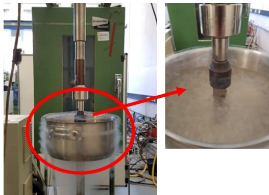
Figure 4.28: Adjusted experimental set-up, to fracture the samples under LN.
