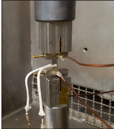
Figure 4.15: 2 mm sample mounted by Kapton covered bolts in the experimental set-up.
