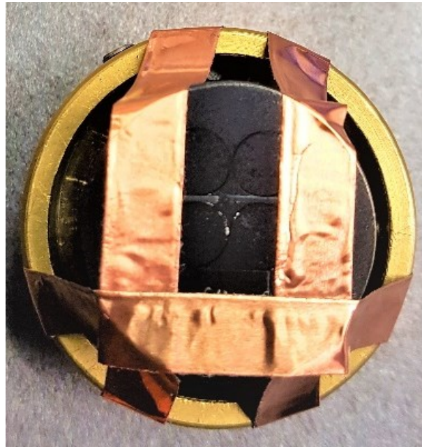
Figure 4.2: Side surface and front surface samples of the 0.5 mm material embedded and ready to be scanned.
