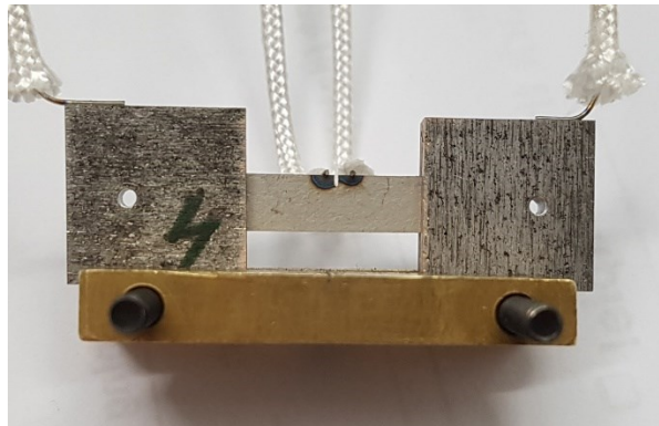
Figure 4.18: Brazed and wired 0.2 mm sample, ready to be tested.
