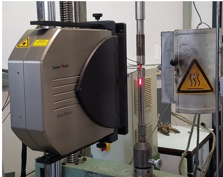
Figure 4.24: Set-up for sample 3_2mm tested at 250°C; on the right the tubular heating chamber of the furnace can be seen.
