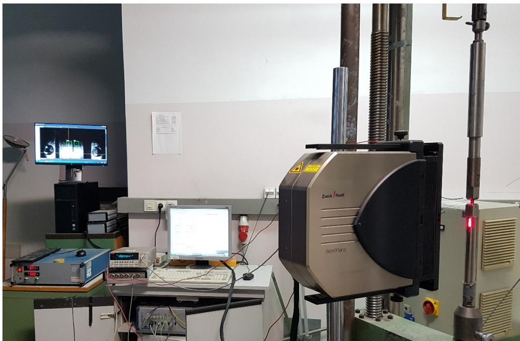
Figure 4.19: Experimental set-up I, almost complete as deployed in one of the experiments. The laser extensometer is pointing at the sample for measuring the displacement of the sample. The sample is fixed within a long linkage, which leaves enough space for later furnace mounting (the furnace is not placed within the frame of the image).
