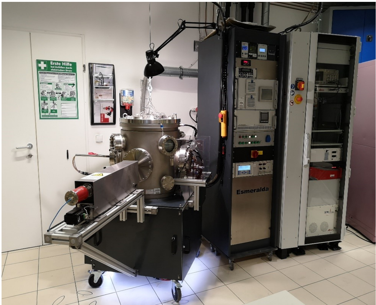
Fig. 3.1: Photograph of deposition system “Esmeralda” used in this work.
