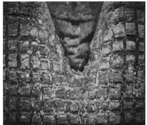
Anodic Indenter - Clay compaction around indenter
