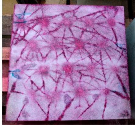
Figure 20 Crack pattern of several irradiated spots. (Hartlieb and Grafe 2017)
