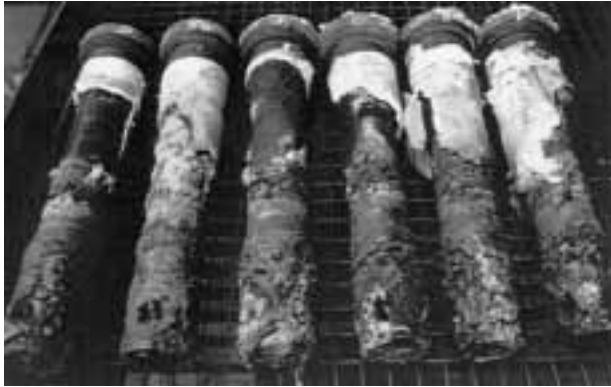
Fig. 5. External view of clogged submerged entry nozzles 22
