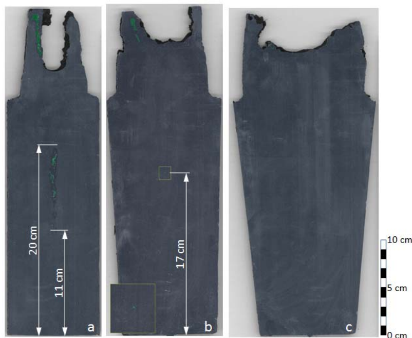
Figure 4. Experimental results of the cast ingots (a: 0^\circ taper; b: 5^\circ taper; c: 10^\circ taper).
