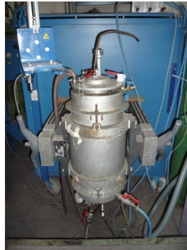
Figure 4. a) Schematic illustration of the test arrangement and b) photograph of the Tammann furnace used for laboratory experiments.
