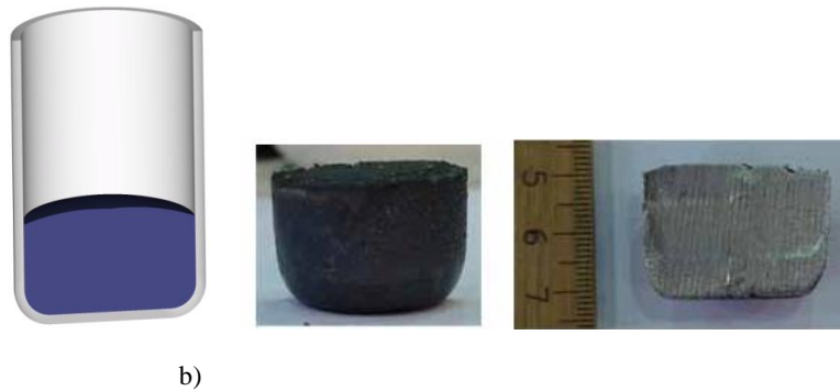
Figure 5. a) Schematic section through the crucible and the sample b) photograph of a remelted sample and the vertical section of the sample.
