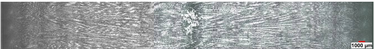
Fig. 3: Primary etching of a thin slab (0.06 wt.-% C, 80 mm thickness) from ESP Arvedi-masterplant.
