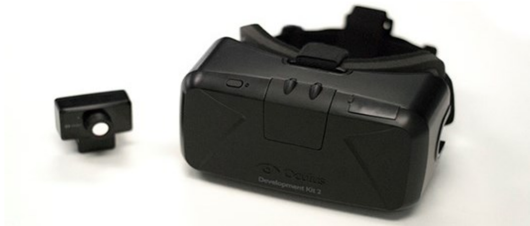
Figure 32: Oculus rift developer kit 2 with an additional motion sensor ( http://www.oculus.com/blog/announcing-the-oculus-rift-development-kit-2-dk2/ ; seen: 20.11.2014)
