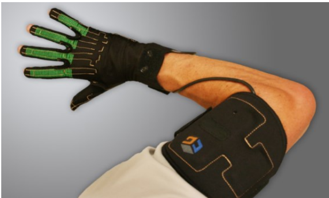
Figure 33: Cyber glove III represents one out of the two possibilities to introduce 3D input technology. ( http://www.cyberglovesystems.com/products/cyberglove-III/overview , seen on: 20.11.2014)
