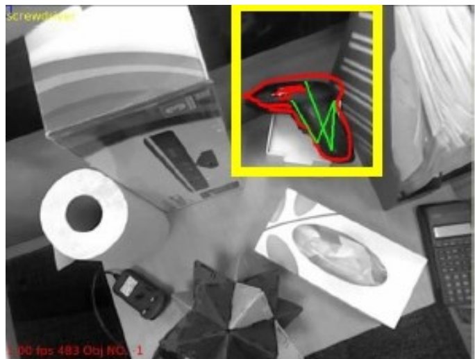
Figure 35: The principle of object identification of the system should work as shown in this picture
