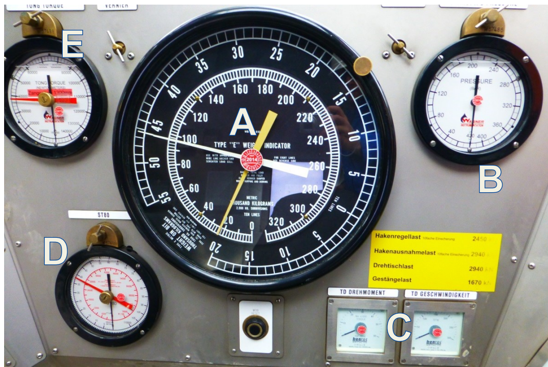
Figure 4: This figure shows the drillers console in front the driller, including the Martin Decker, SPP, TD TQ and TD RPM, tong TQ as well as the iron roughneck TQ
