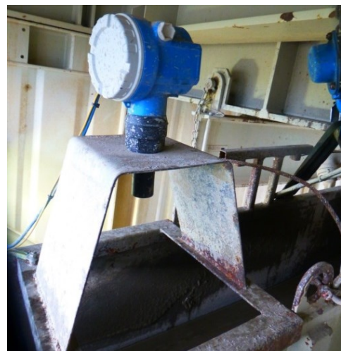
Figure 39: Mud outflow tracking sensor on the RAG Drilling Rig E200. The measurement of the outflow is based on the principle by calculating the flow rate, using the ultra-sonic transit time sensor.
