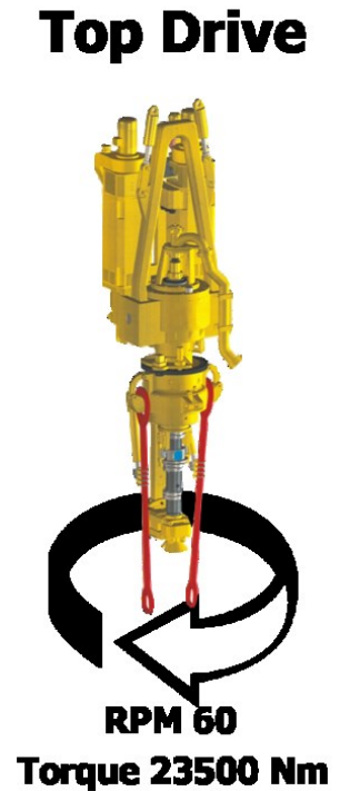
Figure 37: Indicates the turning direction including the RPM and torque reading.
