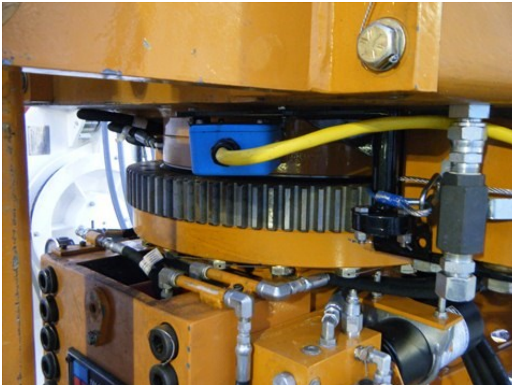
Figure 40: Drill Monitor sensor: rotational and torque measurement ( www.rigsmart.com ; seen on: 24.10.2014)
