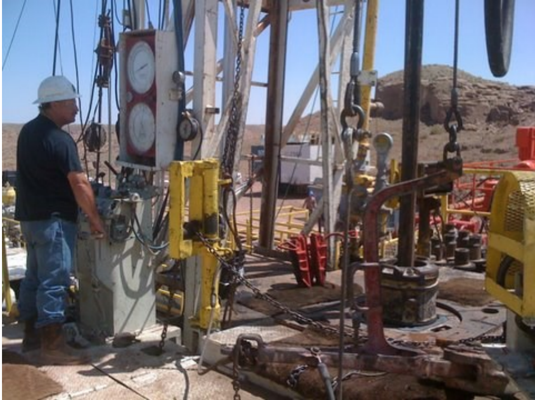
Figure 2: Kelly drilling rig with a simple driller-rig interface. Including a Martin Decker, torque observation gauge and stand pipe pressure manometer.
