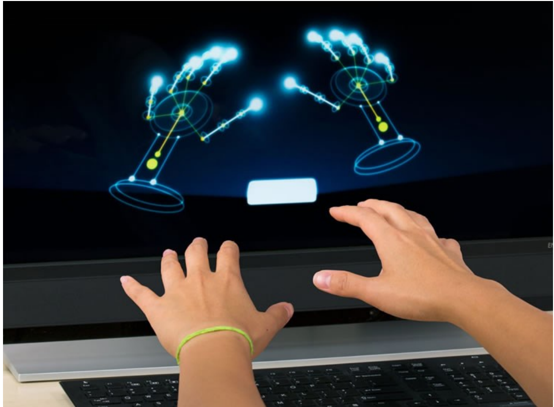
Figure 34: Leap motion demo which indicates the capability of tracking hands and finger motions.
