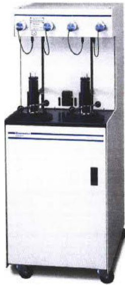
FIGURE 2.1: Autopore IV 9520 mercury injection porosimeter [Peters, 2012]
